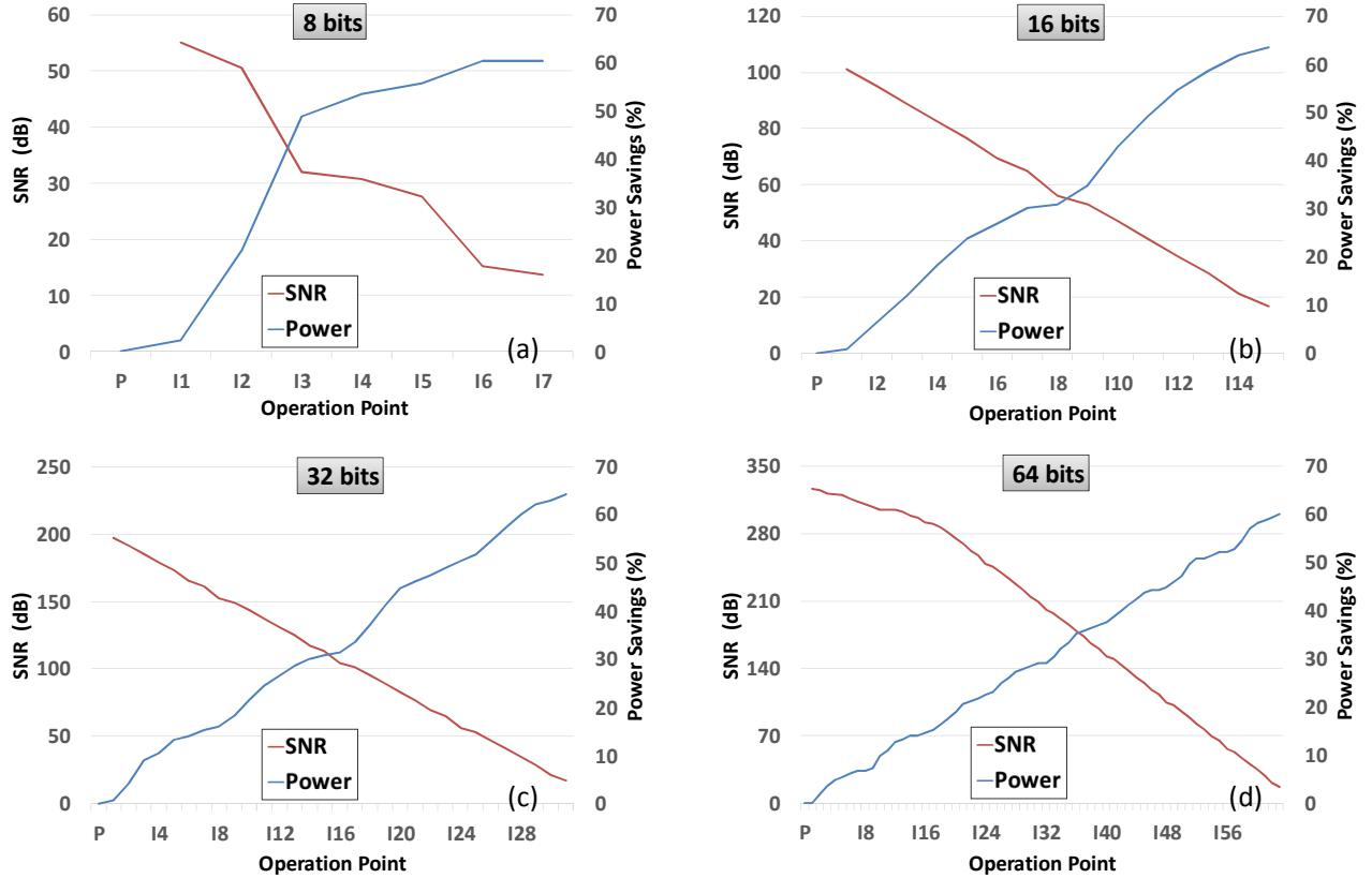
Fig. 3. Power-precision 2PSA evaluations (a) 8-bit adder, (b) 16-bit adder, (c) 32-bit adder and (d) 64-bit adder.
