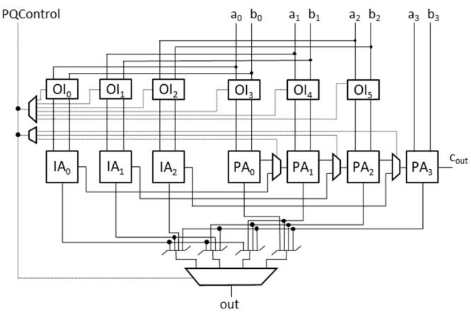
Fig. 1. Block diagram of a 4-bit 2PSA
