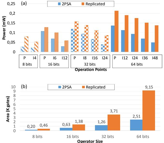
Fig. 4. (a) Power and (b) area comparison between 2PSA and the replicated adders architecture
