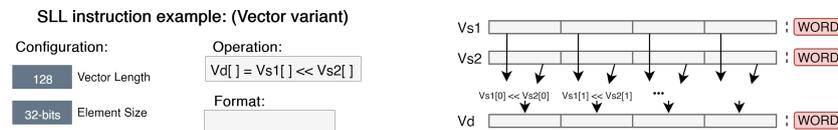
**Figure 4.4:** Shift left logical vector variant operation. Each element of the first source register is shifted by the amount given by the scalar source register. The resulting value is saved in the respective element of the destination register. The example assumes that the vector register length is 128-bits and the element width is a word (32-bits).
