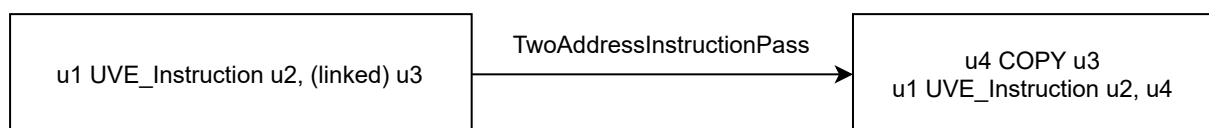
Figure 3.1: Example instruction before and after the two address instruction pass.
