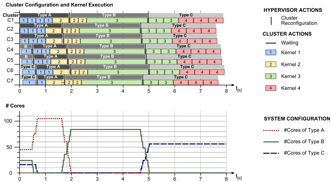
Figure 5.12: Real-time adaptation of the processing architecture, without any a priori knowledge of the computing kernels (Kernel order: 1, 2, 3, 4).
