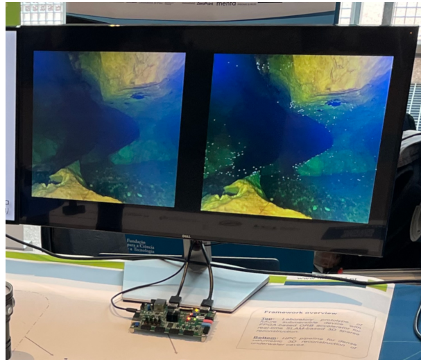
Figure 5.2: Real-time extracted feature overlay demonstration. The two video streams presented side by side are the feeds being streamed to and from the Zybo Z7-20 board (left and right respectively) where the detected features are highlighted in white colour.
